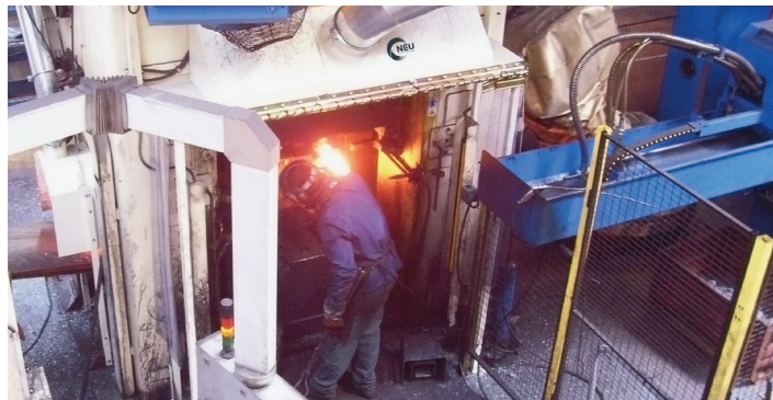
Extraction of graphite dust on forging for press
