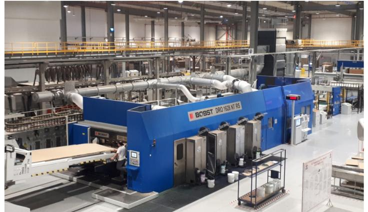
Dust extraction system on converting and printing machines
