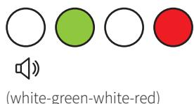
If a terminal device is already in PO mode and a permanently closed tag is held in front of the device, the colour combination shown left is displayed. The device goes into permanently closed mode.
