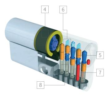
6 3 OF THESE ARE INNOVATIVE ADDITIONAL PAIRS OF PIN TUMBLERS, ARRANGED AXIALLY IN THE SECOND ROW
