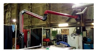
In a shipbuilding company, and especially in the boiler workshop, operators can be exposed to welding fumes released at their workstation.
