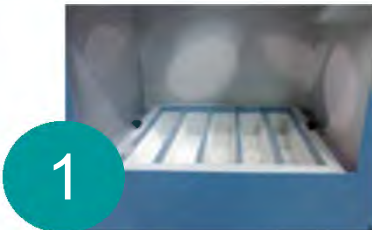
1 Pocket filter designed to ensure collection of as much dust as possible (M6)
