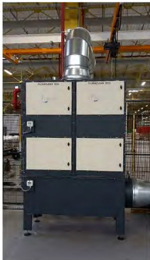
1 Pocket filter designed to ensure collection of as much dust as possible (M6)
