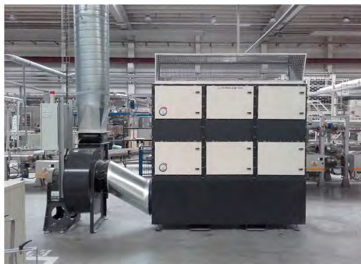
2 3 Second and third high efficiency filtration stages (F8 and E11)
