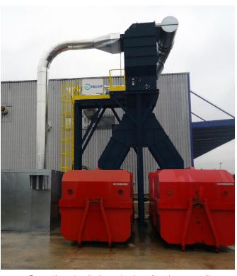
Pneumatic waste collection system in cardboard company with SEPAROJET M and CHOPPERLINE
