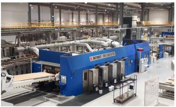
Dust extraction system on converting and printing machines
