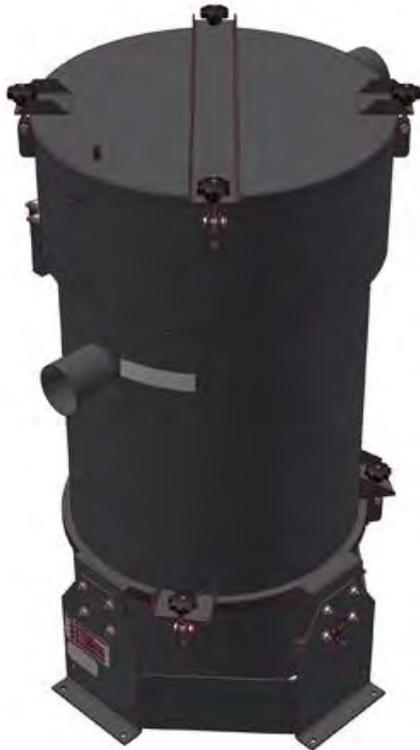
The **NEUMATIC® JK** is a dust collector with filter cartridges. It is a circular filter vessel with filter elements unclogged by the injection of compressed air inside the filter elements. They are specially designed to be integrated in high vacuum suction installations such as floor, machines and workstations cleaning or collection facilities on portable tools (orbital sander or others).
