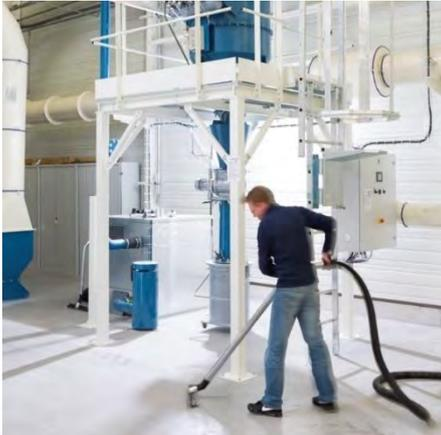
The **NEUMATIC® JE-JR** is a dust collector with automatic cleaning by injection of compressed air and constitutes the major part of a centralised cleaning installation.
