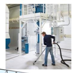
The **NEUMATIC® JE-JR** is a dust collector with automatic cleaning by injection of compressed air and constitutes the major part of a centralised cleaning installation.
